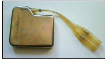
Figure 11.19. ELA Stimulith (l'Électronique Appliquée, Montrouge, France) design. Courtesy Dr. Cristina Tentori, Hospital Juan A. Fernández, Buenos Aires, Argentina).
