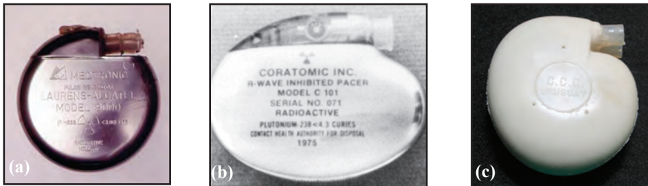
Figure 3.14. Nuclear-powered IPGs manufactured by (a) Medtronic and Laurens-Alcatel , (b) Coratomic , (c) Centro de Construcción de Cardioestimuladores del Uruguay (Courtesy David Prutchi, PhD. )
